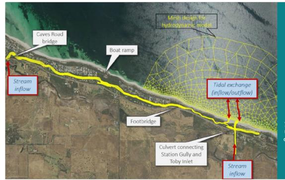
A hydrodynamic model was developed by the Department of Water and Environmental Regulation to assess the different options to increase tidal flushing of the Inlet. The yellow mesh represents the model domain where water depth, salinity, temperature and flow velocity are calculated.
