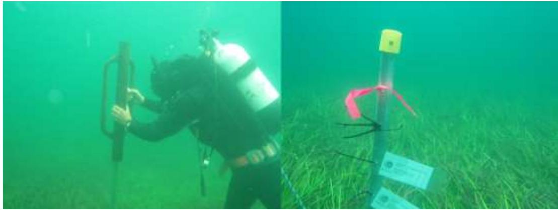
Figure 2: Left: Banging in permanent marker with pole driver. Right: Star picket with cap and plastic coated site label, indicating center of 50 m diameter Keep Watch seagrass site.
