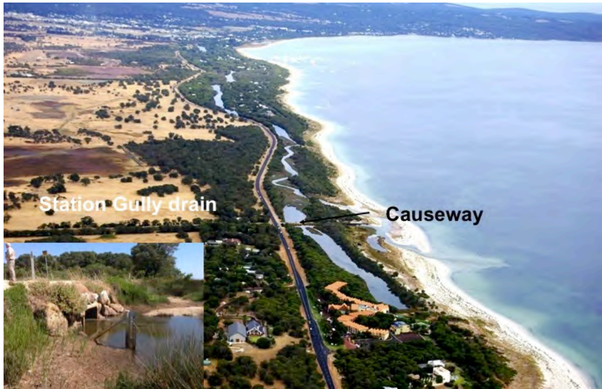
Figure 9: Photo of Toby Inlet showing the Station Gully drain, the flow to the ocean and an insert of the causeway and culvert (Note: at this time there was a channel to the ocean from Toby Inlet on the western side of the causeway).
