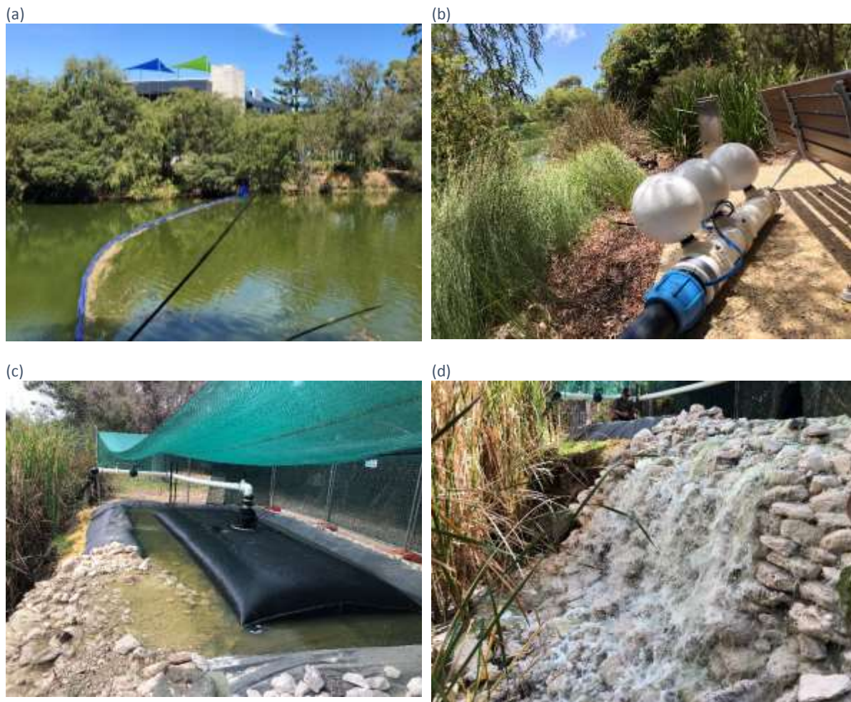
Figure 2. Circulation trial set-up photos showing: (a) PVC separation curtain, (b) submersible pump, (c) the geotextile bag and pond in the outflow area and (d) the rock riffle return to the river.
