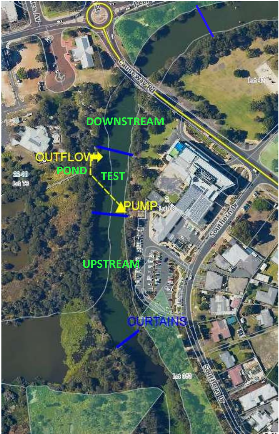
Figure 1. Lower Vasse River circulation trial layout 2019-2020 showing: location of pump, pipe (yellow dashed line) and outflow; separation curtains (blue, approximate location) and water quality monitoring sites (labelled in green).
